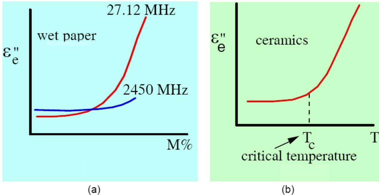
**Fig. 3 Loss factor as a function of (a) the moisture content  $M$  and (b) temperature  $T$**
