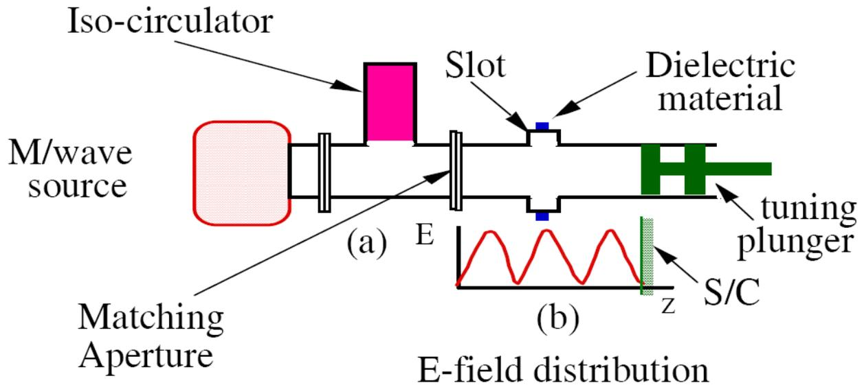
**Fig. 11  $TE_{10n}$  single mode resonant applicator**
