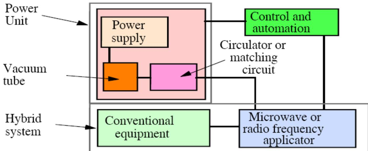
**Fig. 4. Typical microwave heating set-up**
