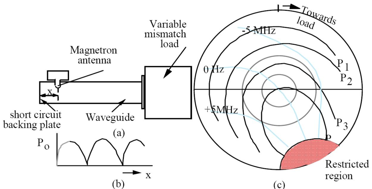
Fig. 6 (a) Waveguide launcher (b) power distribution and (c) Rieke diagram
