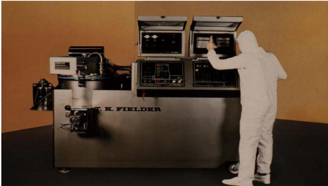
*Fig.12 Combined mixing, granulating and vacuum drying system (Courtesy of NIRO T.K. Fielder Ltd)*
